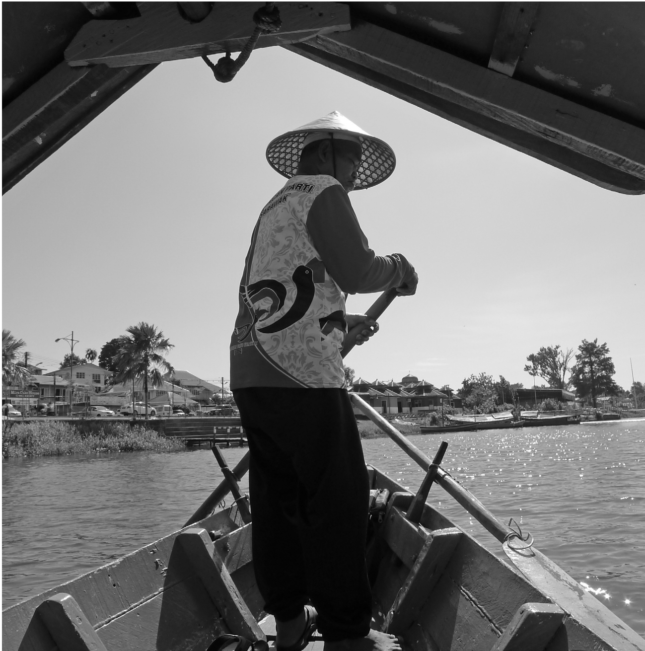
The panambang is a river taxi in Borneo. Two oars in front steer the boat. It is constructed from wood and powered by a small outboard motor attached to the hull in the centre instead of at the rear. Pulling on ropes enables the boatman to start, stop and adjust the engine's throttle. He collects a fixed fare of about one ringgit (22 cents) from one river point to another.
